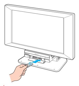
Be sure to hold the Memory Stick with the arrow pointing in the correct direction as you insert it into the slot. To avoid damaging the computer or the Memory Stick, do not force the Memory Stick into the slot if it does not insert smoothly.
